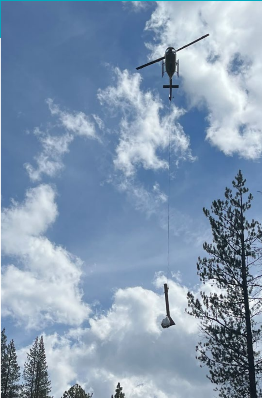
Flying 14ft precipitation gage into Poison Flat
